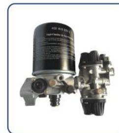
AIR DRYER HL NO.: HL53005 REF NO.: H932 500 007 0 TECHNICAL PARAMETERS: PORT 11: M22x1.5 PORT 12: M12x1.5 PORT 21,22: M22x1.5 VOSS PORT 23,24: M22x1.5 VOSS PORT 25,26: M22x1.5 VOSS
