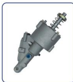
CLUTCH SERVO HL NO.: HL71041 REF NO.: H622107AM TECHNICAL PARAMETERS: DIA: 100mm AIR: M16 × 1.5 HYD: M14 × 1.5 STROKE: 50mm
