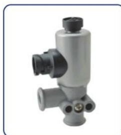
SOLENOID VALVE HL NO.: HL87012 REF NO.: H472 070 639 0 TECHNICAL PARAMETERS: PORT 1,2: M12x1.5 DC 24V
