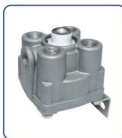
R-12 RELAY VALVE HL NO.: HL82019 REF NO.: H102626 TECHNICAL PARAMETERS: SUPPLY PORTS : 1-NPT1/2 DELIVERY PORTS: 4-NPT1/2 SERVICE PORT: 1-NPT1/4
