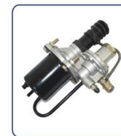
CLUTCH SERVO HL NO.: HL71053 REF NO.: H642-03080 TECHNICAL PARAMETERS: DIA: 70mm AIR: M14 × 1.5 HYD: M12 × 1.5 STROKE: 35mm
