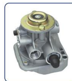
RELAY EMERGENCY VALVE HL NO.: HL82027A REF NO.: H971 002 304 0 TECHNICAL PARAMETERS: PORT 1: M22x1.5 PORT 2: M22x1.5 PORT 1-2: M22x1.5 PORT 4: M22x1.5
