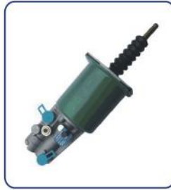
CLUTCH SERVO HL NO.: HL71034 REF NO.: HVG3208 TECHNICAL PARAMETERS: DIA: 100mm AIR: M16 × 1.5 HYD: M14 × 1.5 STROKE: 84mm
