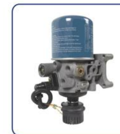
AIR DRYER HL NO.: HL53012 REF NO.: HLA8130 TECHNICAL PARAMETERS: HEAT: 24V PORT 1,12: M22x1.5 PORT 21: M16x1.5 PORT 23: M16x1.5 VOSS PORT 24: M22x1.5 VOSS
