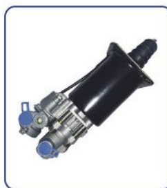
CLUTCH SERVO HL NO.: HL71004 REF NO.: H970 051 114 0 TECHNICAL PARAMETERS: DIA: 75mm AIR: M16 x 1.5 HYD: M14 x 1.5 STROKE: 67mm
