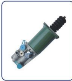
CLUTCH SERVO HL NO.: HL71033/71033A REF NO.: HVG3200 HVG3204(A) TECHNICAL PARAMETERS: DIA: 75mm AIR: M16 × 1.5 HYD: M14 × 1.5 STROKE: 84mm
