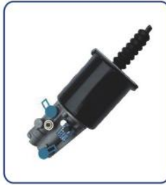
CLUTCH SERVO HL NO.: HL71035/71035A REF NO.: HVG3213 HVG3229(A) TECHNICAL PARAMETERS: DIA: 100mm AIR: M16 × 1.5 HYD: M14 × 1.5 STROKE: 84mm
