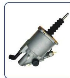
CLUTCH SERVO HL NO.: HL71048 REF NO.: H627052AM TECHNICAL PARAMETERS: DIA: 100mm AIR: M22 × 1.5 VOSS HYD: M14 × 1.5 STROKE: 85mm
