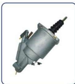
CLUTCH SERVO HL NO.: HL71040 REF NO.: H627479AM TECHNICAL PARAMETERS: DIA: 100mm AIR: M16 × 1.5 HYD: M14 × 1.5 STROKE: 58mm
