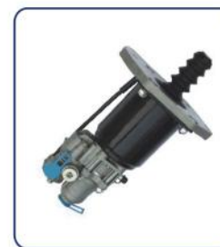
CLUTCH SERVO HL NO.: HL71010 REF NO.: H970 051 151 0 TECHNICAL PARAMETERS: DIA: 85mm AIR: M16 x 1.5 HYD: M14 x 1.5 STROKE: 65mm
