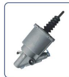
CLUTCH SERVO HL NO.: HL71050/71050A REF NO.: H628275AM H628259AM(A) TECHNICAL PARAMETERS: DIA: 100mm AIR: M16 × 1.5 HYD: M14 × 1.5 STROKE: 85mm
