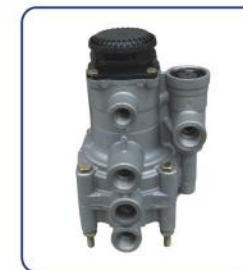
TRAILER CONTROL VALVE HL NO.: HL85003 REF NO.: H973 009 300 0 TECHNICAL PARAMETERS: PORT 11,12,22: M22x1.5 VOSS PORT 41,42: M22x1.5 VOSS PORT 43: M16x1.5 VOSS PREDOMINANCE: 0.2BAR COMMENT: WITH SILENCER
