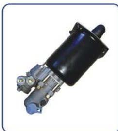
CLUTCH SERVO HL NO.: HL71068 REF NO.: H970 051 125 0 TECHNICAL PARAMETERS: DIA: 102mm AIR: M16 x 1.5 HYD: M14 x 1.5 STROKE: 70mm
