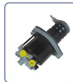
CLUTCH SERVO HL NO.: HL71012 REF NO.: H970 051 158 0 TECHNICAL PARAMETERS: DIA: 102mm AIR: M16 x 1.5 HYD: M14 x 1.5 STROKE: 75mm
