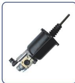
CLUTCH SERVO HL NO.: HL71027/71027A REF NO.: H970 510 446 0 H970 051 412 0(A) TECHNICAL PARAMETERS: DIA: 102mm AIR: M22 × 1.5 VOSS HYD: M14 × 1.5 STROKE: 85mm
