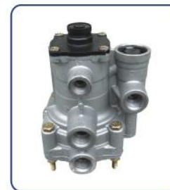
TRAILER CONTROL VALVE HL NO.: HL85001 REF NO.: H973 009 001 0 TECHNICAL PARAMETERS: PORT 11,12,22,41,42: M22x1.5VOSS PORT 43: M16x1.5 VOSS PREDOMINANCE: 0.2BAR
