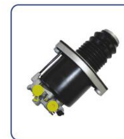
CLUTCH SERVO HL NO.: HL71013 REF NO.: H970 051 159 0 TECHNICAL PARAMETERS: DIA: 102mm AIR: M16 x 1.5 HYD: M14 x 1.5 STROKE: 75mm
