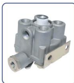
R-14 RELAY VALVE HL NO.: HL82017 REF NO.: H103028 TECHNICAL PARAMETERS: SUPPLY PORTS: 1-NPT1/2 DELIVERY PORTS: 4-NPT1/2 SERVICE PORT: 1-NPT1/4 BALANCE PORT : 1-NPT1/8
