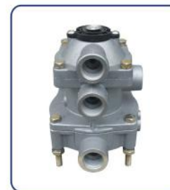
TRAILER CONTROL VALVE HL NO.: HL85005 REF NO.: H973 002 007 0 TECHNICAL PARAMETERS: PORTS 1,2: M22x1.5 PORTS 41,42,43: M22x1.5 PREDOMINANCE: 0.6BAR PREDOMINANCE: 0BAR-ADJUSTABLE
