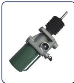
CLUTCH SERVO HL NO.: HL71031 REF NO.: HAPGA16XX TECHNICAL PARAMETERS: DIA: 63.5mm AIR: 1/8-27 NPTF HYD: 7/16-20 NPTF STROKE:
