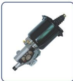
CLUTCH SERVO HL NO.: HL71019 REF NO.: H970 051 402 0 TECHNICAL PARAMETERS: DIA: 102mm AIR: M16 × 1.5 HYD: M14 × 1.5 STROKE: 25.2mm
