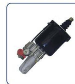
CLUTCH SERVO HL NO.: HL71017 REF NO.: H970 051 192 0 TECHNICAL PARAMETERS: DIA: 100mm AIR: M16 x 1.5 HYD: M14 x 1.5 STROKE: 58.5mm
