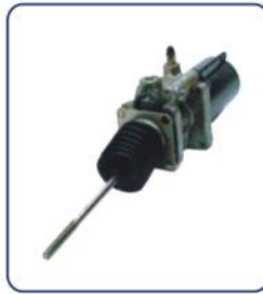
CLUTCH SERVO HL NO.: HL71032 REF NO.: HAPGA1610/4 TECHNICAL PARAMETERS: DIA: 75mm AIR: M16 × 1.5 HYD: STROKE: 67mm
