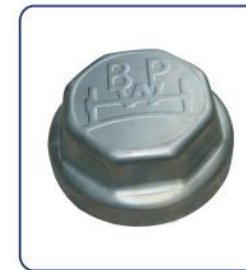
HUB COVER HL NO.: HL46005 TYPE: 14T TECHNICAL PARAMETERS: SIZE: 148x2 Inside Thread
