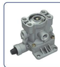
RELAY EMERGENCY VALVE HL NO.: HL82024 REF NO.: H971 002 152 0 TECHNICAL PARAMETERS: PORT 1: M22x1.5 PORT 1-2=M22x1.5 PORT 4=M16x1.5 PORT 2=4-M16x1.5+1-M22x1.5
