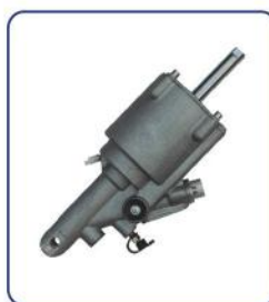
CLUTCH SERVO HL NO.: HL71047 REF NO.: H626639AM TECHNICAL PARAMETERS: DIA: 95mm AIR: M16 × 1.5 HYD: M14 × 1.5 STROKE: 70mm
