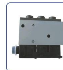
SOLENOID VALVE HL NO.: HL87028A/87028B REF NO.: H3944716(A) H3944717(B) TECHNICAL PARAMETERS: PORT 1,21,22: M22x1.5 DC 24V
