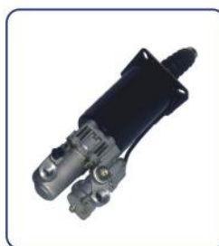
CLUTCH SERVO HL NO.: HL71009 REF NO.: H970 051 137 0 TECHNICAL PARAMETERS: DIA: 75mm AIR: M16 x 1.5 HYD: M14 x 1.5 STROKE: 85mm
