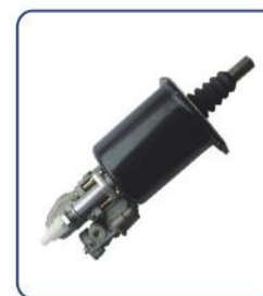
CLUTCH SERVO HL NO.: HL71014 REF NO.: H970 051 164 0 TECHNICAL PARAMETERS: DIA: 102mm AIR: M16 x 1.5 HYD: M14 x 1.5 STROKE: 85mm
