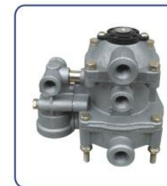
TRAILER CONTROL VALVE HL NO.: HL85004 REF NO.: H973 002 521 0 TECHNICAL PARAMETERS: PORT 11,12,22: M16x1.5 PORT 41,42,43: M16x1.5 PREDOMINANCE: 0.2 PREDOMINANCE ADJUSTABLE: YES
