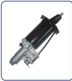
CLUTCH SERVO HL NO.: HL84023 REF NO.: H970 051 435 0 TECHNICAL PARAMETERS: DIA: 75mm AIR: M16 × 1.5 HYD: M14 × 1.5 STROKE: 85mm
