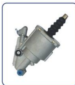
CLUTCH SERVO HL NO.: HL71043 REF NO.: H622199AM TECHNICAL PARAMETERS: DIA: 100mm AIR: M16 × 1.5 HYD: M14 × 1.5 STROKE: 70mm
