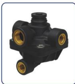
RELAY VALVE HL NO.: HL82010 REF NO.: H973 006 000 0 TECHNICAL PARAMETERS: PORT 1: M22x1.5 PORT 2: M16x1.5 PORT 4: M16x1.5
