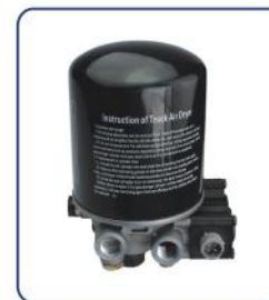
AIR DRYER HL NO.: HL53007 REF NO.: H432 425 101 0 TECHNICAL PARAMETERS: HEAT: 24V PORT 1,21: M22x1.5 VOSS PORT 4: M12x1.5 PORT 12: M12x1.5
