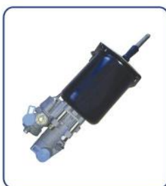
CLUTCH SERVO HL NO.: HL71008/71008A REF NO.: H970 051 132 0 H970 051 170 0(A) TECHNICAL PARAMETERS: DIA: 102mm AIR: M16 x 1.5 HYD: M14 x 1.5 STROKE: 85mm
