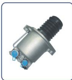
CLUTCH SERVO HL NO.: HL71038 REF NO.: HVG3361 TECHNICAL PARAMETERS: DIA: 102mm AIR: M16 × 1.5 HYD: M14 × 1.5 STROKE: 70mm
