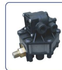
RELAY EMERGENCY VALVE HL NO.: HL82023 REF NO.: H28600 TECHNICAL PARAMETERS: SUPPLY PORT: 1-NPT3/8 CONTROL PORT: 1-NPT1/4 RESERVOIR PORT: 1-NPT3/4 SERVICE BRAKE PORTS: 4-NPT3/8 SPRING BRAKE PORTS: 2-NPT3/8
