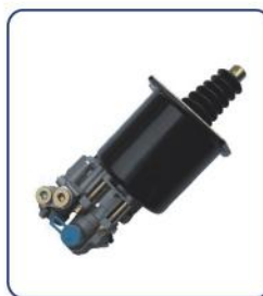
CLUTCH SERVO HL NO.: HL71002 REF NO.: H970 051 107 0 TECHNICAL PARAMETERS: DIA: 102mm AIR: M16 x 1.5 HYD: M14 x 1.5 STROKE: 58.5mm
