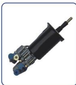
CLUTCH SERVO HL NO.: HL71003 REF NO.: H970 051 111 0 TECHNICAL PARAMETERS: DIA: 75mm AIR: M16 x 1.5 HYD: M14 x 1.5 STROKE: 85mm
