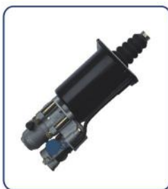
CLUTCH SERVO HL NO.: HL71001 REF NO.: H970 051 102 0 TECHNICAL PARAMETERS: DIA: 75mm AIR: M16 x 1.5 HYD: M14 x 1.5 STROKE: 67mm
