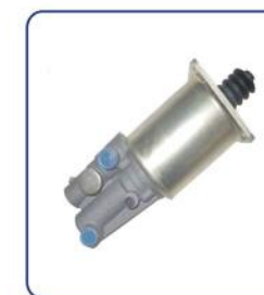
CLUTCH SERVO HL NO.: HL71059 REF NO.: HWG9114230023 TECHNICAL PARAMETERS: DIA: 90mm × 22mm AIR: M16 × 1.5 HYD: M14 × 1.5 STROKE: 67mm
