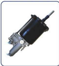
CLUTCH SERVO HL NO.: HL71021A REF NO.: H970 051 407 0 TECHNICAL PARAMETERS: DIA: 102mm AIR: M16 × 1.5 HYD: M14 × 1.5 STROKE: 85mm
