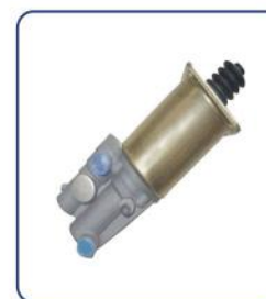
CLUTCH SERVO HL NO.: HL71058 REF NO.: HWG9114230022 TECHNICAL PARAMETERS: DIA: 75mm × 22mm AIR: M16 × 1.5 HYD: M14 × 1.5 STROKE: 75mm
