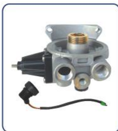
AIR DRYER SEAT HL NO.: HL52002 REF NO.: H432 410 600 2 TECHNICAL PARAMETERS: HEAT: 24V CONN: M27x1 PORT 1,21: M22x1.5 PORT 22: M12x1.5
