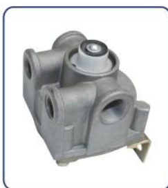
R-12H RELAY VALVE HL NO.: HL82015 REF NO.: H103009 TECHNICAL PARAMETERS: SUPPLY PORTS: 2-NPT3/4 DELIVERY PORTS: 2-NPT1/2 SERVICE PORT: 1-NPT1/4
