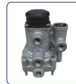
TRAILER CONTROL VALVE HL NO.: HL85002 REF NO.: H973 009 010 0 TECHNICAL PARAMETERS: PORT 11,12,22: M16x1.5 PORT 41,42,43: M16x1.5 PREDOMINANCE: 0.4BAR COMMENT: WITH SILENCER
