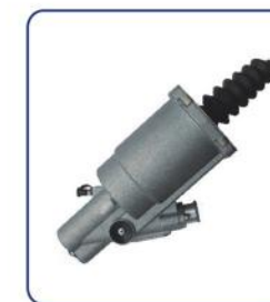
CLUTCH SERVO HL NO.: HL71051/71051A REF NO.: H628276AM H628277AM(A) TECHNICAL PARAMETERS: DIA: 80mm AIR: M16 × 1.5 HYD: M14 × 1.5 STROKE: 85mm
